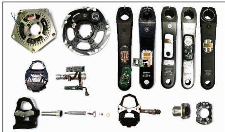
Cycling power meters, from all the major manufactureres, were taken apart.
